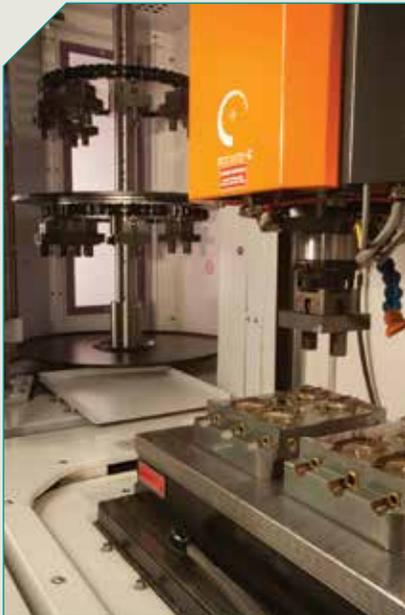
The advanced IQ generator technology of the GF AgieCharmilles FORM 350 SP sinker EDM gives Janler increased speed and superior surface finishes while also virtually eliminating electrode wear to reduce electrode material costs.
