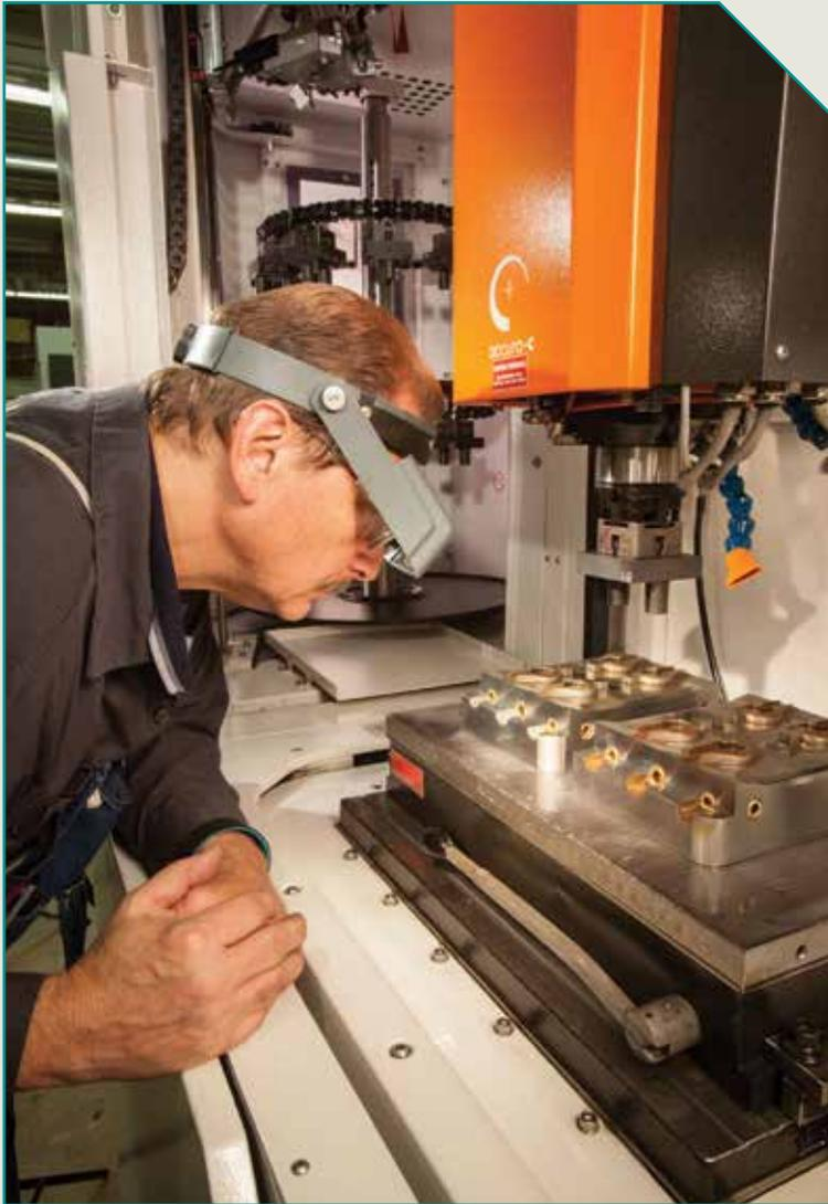
Janler moldmaker and EDM expert Karle Lang inspects the intricate mold details produced on the shop's GF AgieCharmilles FORM 350 SP sinker EDM.
